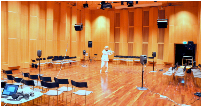
Fig. 5: Rehearsal before the performance at Norwegian Academy of Music. Parts of the computer and mixer setup to the left, the camera hangs in the ceiling, and the 8 loudspeakers are placed in two squares around the quadratic stage area.
